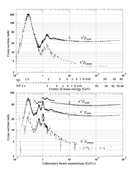
Figure 37.20: Total and elastic cross sections for  $\pi^{\pm}p$  and  $\pi^{\pm}d$  (total only) collisions as a function of laboratory beam momentum and total center-of-mass energy. Corresponding computer-readable data files may be found at http://pdg.lbl.gov/xsect/contents.html (Courtesy of the COMPAS Group, IHEP, Protvino, Russia, August 1999.)
